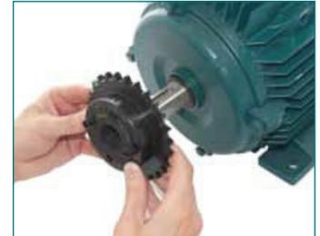
INSERT SCREWS AND LOCATE ON SHAFT
