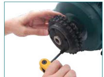
REMOVING A TAPER LOCK BUSH
