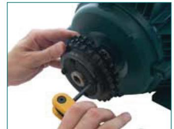
TIGHTEN SCREWS ALTERNATELY
